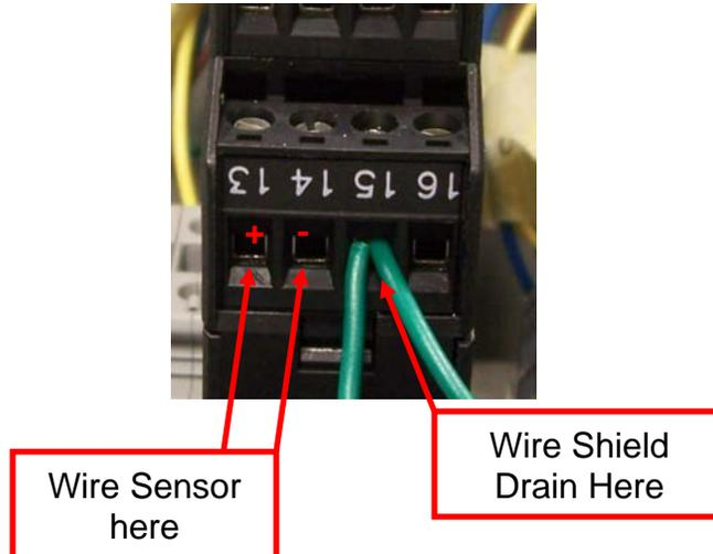
**Figure 5 – Input Wiring**
